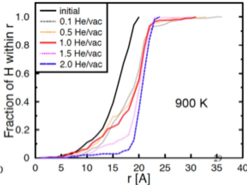
*Calculated fraction of hydrogen that is trapped in the vicinity of a 2 nm radius He bubble in tungsten at 900 K (B.D. Wirth).*
