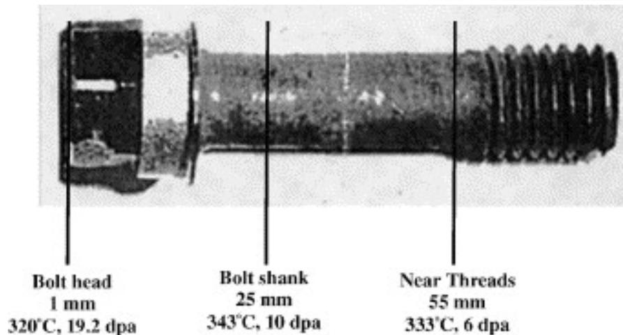
Baffle-former bolt removed from Tihange-1 (Belgium) pressurized water reactor
