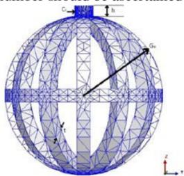
**FIG. 1.** A sample to mesh structures of the 6 vertical ring cathode
