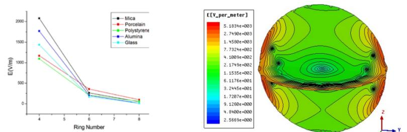
**FIG. 5.** Maximal E field at the middle of grid with respect to the ring number (left) and Electric fields with horizontal and vertical components in the cases of A (right).
