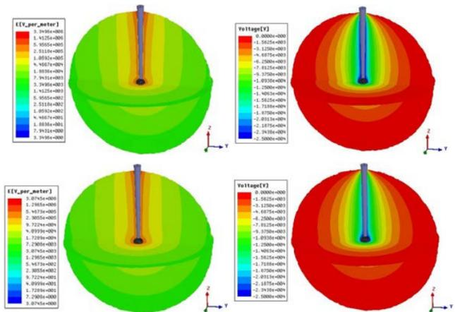
**FIG. 3.** Electric field E and potential  $\phi$  surfaces for alumina (above), glass (below) for the inner grid structure including 8 vertical rings.
