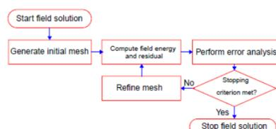
After E is calculated, it produces solution files and performs an error analysis. In the adaptive analysis, it refines the tetrahedrons with the highest error, and continues solving until the stopping criterion is met.
